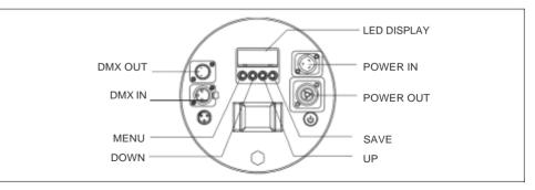
Connect the provided XLR cable to the female 3-pin XLR output of your controller and the other side to the male 3-pin XLR input of the moving head. You can chain multiple Moving head together through serial linking. The cable needed should be two core, screened cable with XLR input and output connectors. Please refer to the diagram below. DMX-512 connection with DMX terminator.
